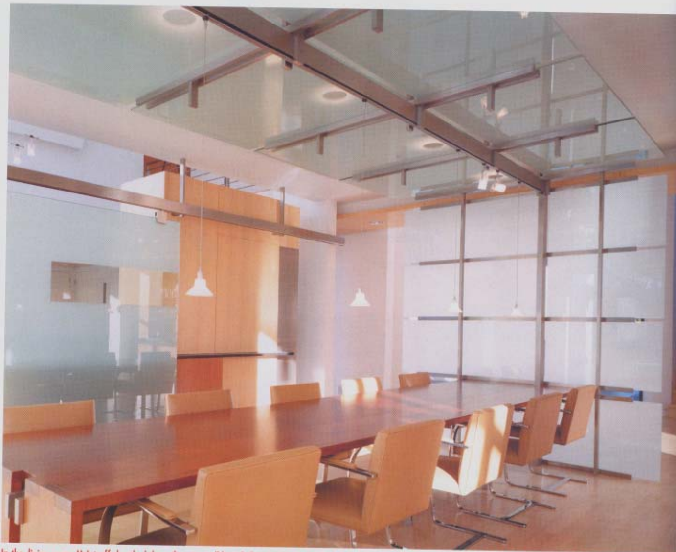
In the dining room, McInturff sheathed the ceiling in sandblasted glass punctuating it with light (above). A rolling screen of sandblasted glass opens from the dining room to reveal the kitchen (opposite).
